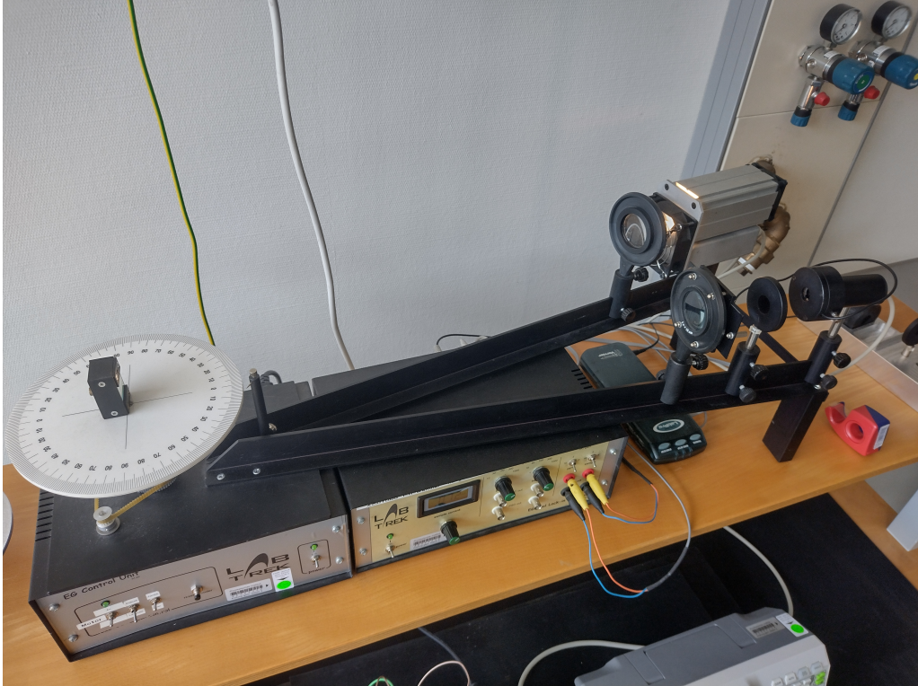
Figure 1: Setup for the band gap measurements
