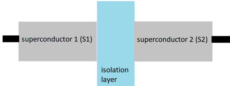
Figure 1: Isolator surrounded by two identical superconductors (Josephson contact)<sup>[4]</sup>
