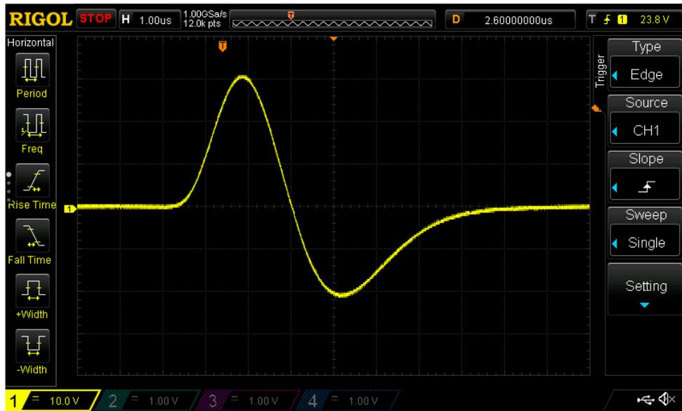
**Figure 7:** The  $^{22}\text{Na}$ -signal detected by the NaI scintillator as given out by the bipolar output of the main amplifier. The coarse gain was set to 20 and the gain to 2, which results in an amplification factor of 14.
