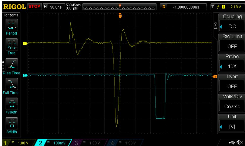
**Figure 12:** The  $^{22}\text{Na}$ -signal output of both the NaI scintillator single channel analyzer (yellow) and the plastic scintillator single channel analyzer (blue).
