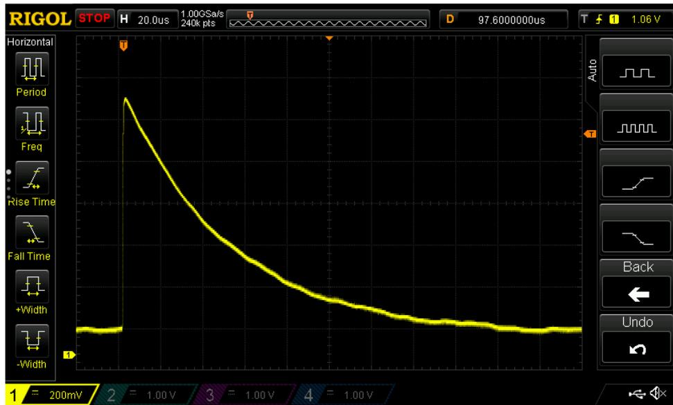
**Figure 5:** The  $^{22}\text{Na}$ -signal detected by the NaI scintillator as given out by the preamplifier. The expected exponential shape is clearly visible.
