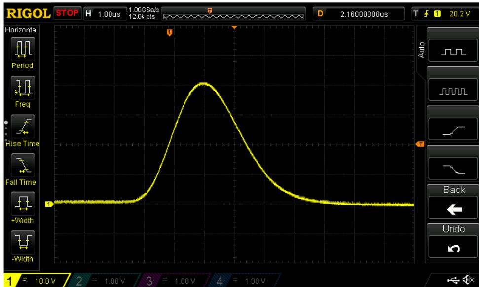
**Figure 6:** The  $^{22}\text{Na}$ -signal detected by the NaI scintillator as given out by the unipolar output of the main amplifier. The coarse gain was set to 20 and the gain to 2, which results in an amplification factor of 14.
