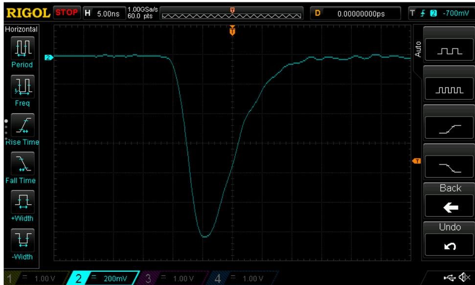
**Figure 9:** The  $^{22}\text{Na}$  detected by the plastic scintillator as given out by the preamplifier. The expected shape (described in [section 3](#)) is clearly visible.
