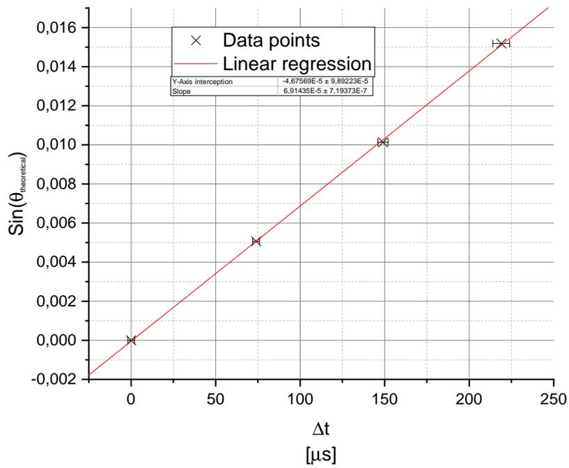
Figure 15: The linear regression for the reference grating with the ultrasound cell.  $\Delta t$  is given in  $\mu s$
