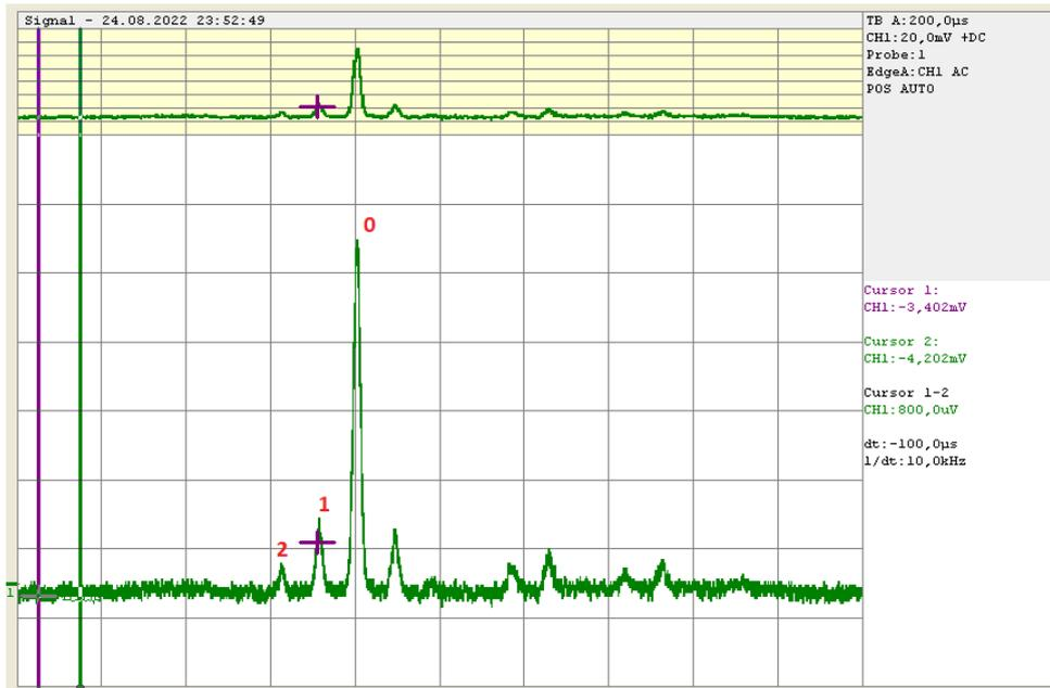
Fig. 23: Screenshot of the oscilloscope for counting the orders of the maxima for the third grating. The  $x$ -axis is the time-axis and the  $y$ -axis the intensity of the interference pattern. In red the two visible peaks are enumerated.
